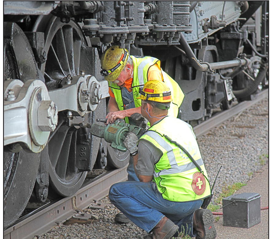
Adding grease to the bearings on locomotive 5511, an engine that had hardly been moved in the last 50 years. – Photo © 2022 Dave Schaaf.
